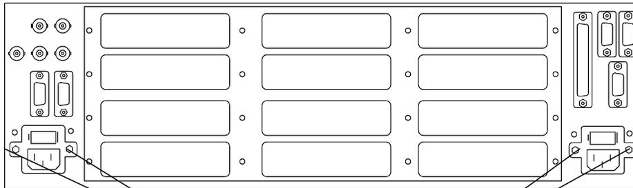
Position of PSU fixing screws
