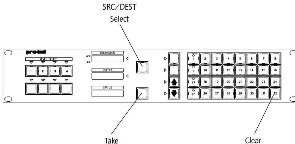
The operation of this panel is identical to that of a Normal 6276 X-Y panel but has the option of being able to configure AUD parameters and trigger type for sources as well as being able to unprotect destinations set from another panel if <PROTECT> assigned.
