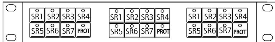
To protect a destination association simply select the desired source association and then press the <PROTECT> button. The protect lamp will light if at least one controllable level in the destination association is protected. When the protect lamp is lit further crosspoint selections on this destination association can be made but crosspoints will only take on the unprotected levels.
